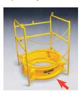
Constructed of rugged, lightweight Polyethylene with bright yellow material that resists fading. Will fit 27", 30" and 32" diameter manholes with an inflatable seal that ensures a watertight seal. Designed with 4-outrigger support gussets that stabilize the shield and is 12" tall to keep water and mud out of manhole as you work. Can be used with Allegro guard rail.
