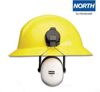
All-purpose lateral impact hard hat with foam liner, HDPE outer shell grooved for rigidity, rain trough and accessory slots. Choice of unique quick fit or ratchet suspension, both with forehead comfort band and crown pad, offering workers greater choice and comfort. Both suspensions feature a 4-point nylon web cradle with three-level height adjustment. ANSI Type II Class E and CSA Type 2 Class E
