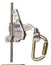
imposed on the ladder structure Locked on for hands-free movement! The swiveling Lad-Saf® sleeve, attached by carabiner to your Delta No-Tangle™ harness, prevents falls by locking onto the cable. It is easily attached or removed anywhere along the cable and automatically follows as you climb or descend
