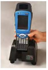
i-Safe™ is exclusive to DBI-SALA and provides a multitude of benefits for the safety conscious. It uses Radio Frequency Identification (RFID) technology to provide quick access to inspection, inventory and information. The inspection feature allows the user to access predetermined questions to inspect and record the inspection without accessing files or notes through the use of a hand-held PC. The system is paperless and reduces the time of inspecting and recording inspections by well over 30%.
